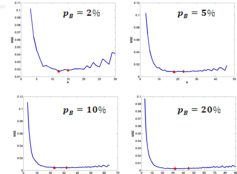
$$k = \left\lceil \frac{\frac{2}{3} \sqrt{p_B \cdot n} + 2}{|\widehat{\mu}_1 - \widehat{\mu}_0|^{1.4}} \right\rceil \quad \begin{array}{c} \text{red arrow} \\ \longrightarrow \end{array}$$
