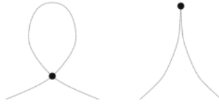
Figure 13.5. Typical singular points: (left) self-intersection, (right) cusp.
